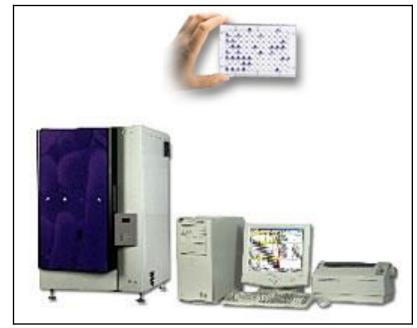
Absorbance was measured with a Dynatech MR-700 microtiter plate reader using Microlog 2N®software (Biolog).
